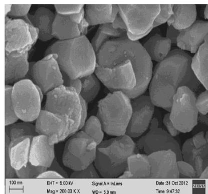
Fig 2: SEM images of (1-x) Ni<sub>0.5</sub>Cu<sub>0.3</sub>Mg<sub>0.2</sub>Fe<sub>2</sub>O<sub>4</sub>+(x) BaTiO<sub>3</sub> for x=0.0
