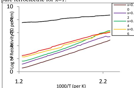
**Fig.4** Variation of dc resistivity ( $\log \rho$ ) with temperature ( $1000/T$ ) for  $(1-x) Ni_{0.5}Cu_{0.3}Mg_{0.2}Fe_2O_4 + (x) BaTiO_3$
