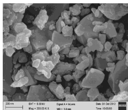
Fig 3: SEM images of (1-x) Ni<sub>0.5</sub>Cu<sub>0.3</sub>Mg<sub>0.2</sub>Fe<sub>2</sub>O<sub>4</sub>+(x) BaTiO<sub>3</sub> for x=0.2
